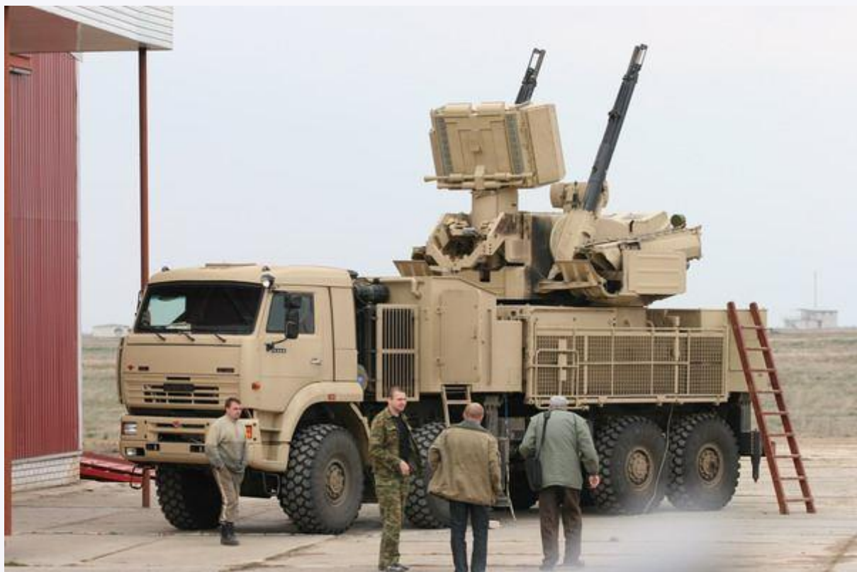
Figure 4: Iraq owns the Russian Pantsir-S1, a mobile short-to-medium-range air defense system designed to protect key assets from aircraft, drones, and precision-guided munitions. Credit: Global Military Review .
